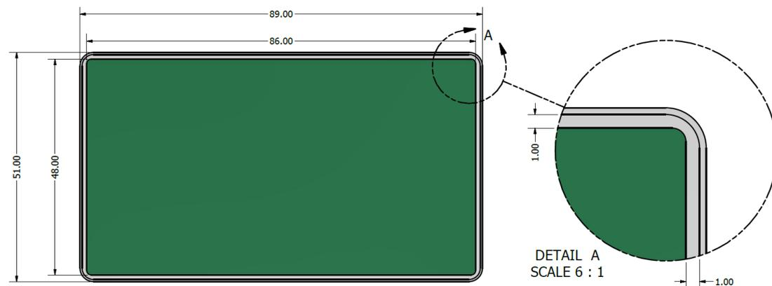
Figure 10 PCB and device enclosure dimensions
