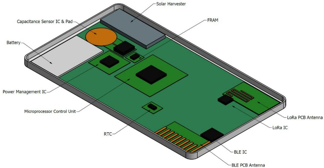
Figure 4 ASSC conceptual core system
