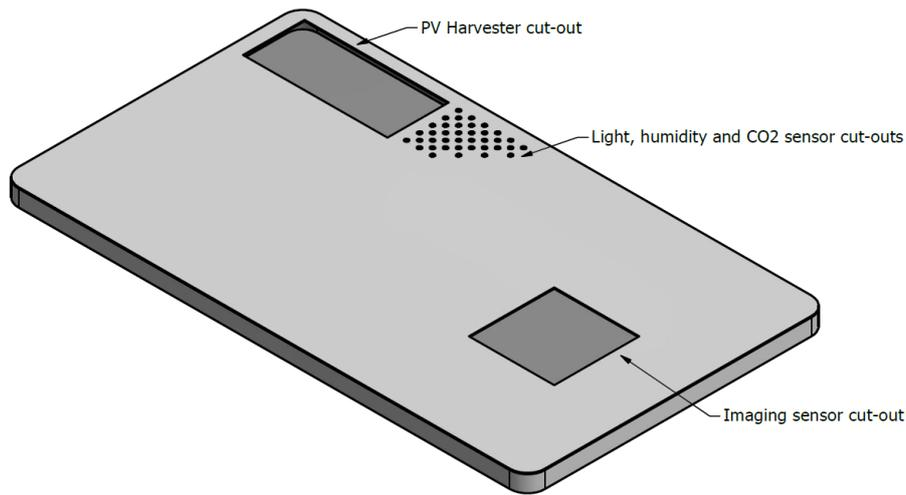
Figure 11 Enclosure openings for sensors
