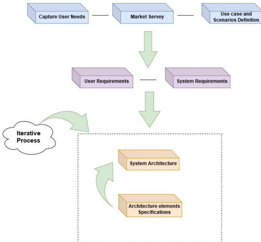
Figure 1 Definition and design process
