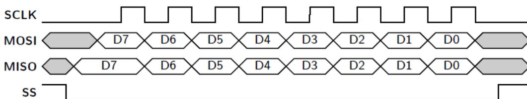
Figure 7 SPI frame
