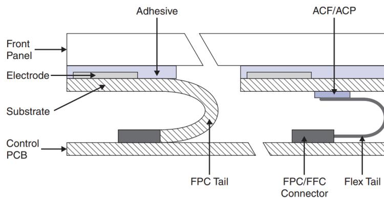
Figure 13 Secondary substrate method of the capacitive sensor [5]
