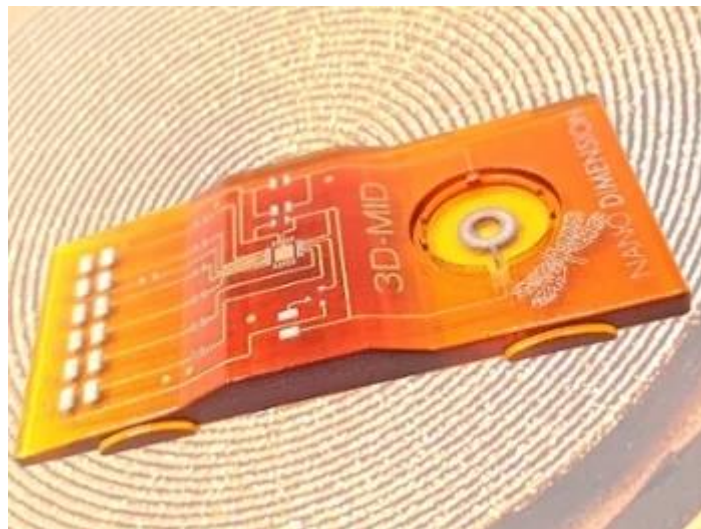
Figure 33 3D-printed non-planar design ready to host electronic parts
