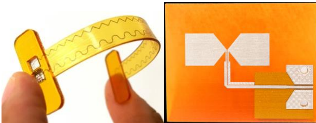
Figure 32 Rigid-flexible design (left), antenna (right)
