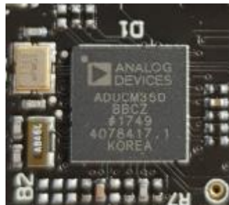
Figure 7 ADUCM350 microcontroller with essential components, size 15x17mm
