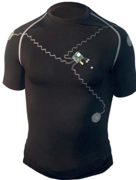
Figure 42 Shirt with electronics, snap fasteners for the battery and embroidered electrodes and conductor [114]
